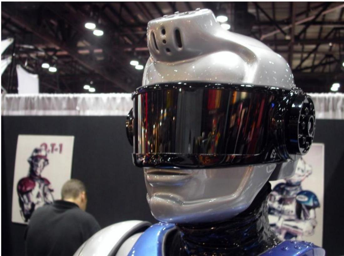
**Panoramic Visor integrated into the head design to allow the Operator clear view of his surroundings! Also note air vents in upper portion of the head, as well as pinhole full color Video Camera!**
